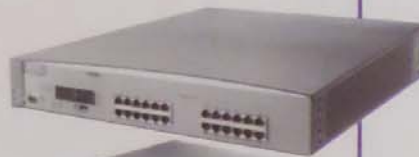
HP ProCurve Switch 2424M
